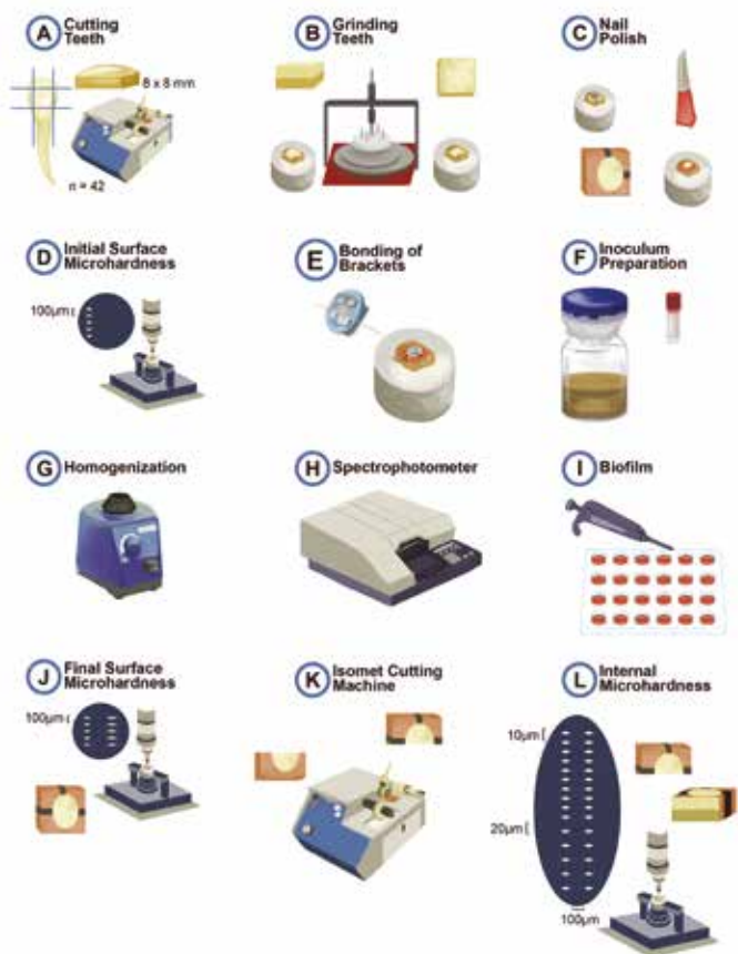
Figure 1. Schematic representing the laboratory stages developed.
