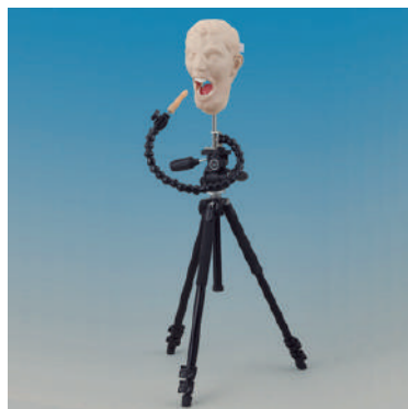
Figura 1. Fantoma radiográfico de adulto (Dental X-Ray Simulator Manikin, Tripod Pedo X-ray Manikin Set, NISSIN DENTAL PRODUCTS INC).
